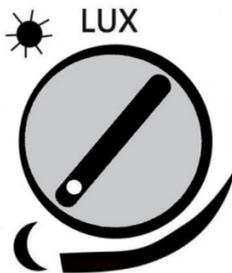
The LUX Adjusting Knob (9) tells the sensor the level of darkness that must be reached before the Light turns on.
